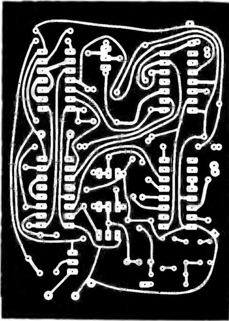
Fig. 3. Actual-size etching and drilling guide for a suitable printed circuit board.
